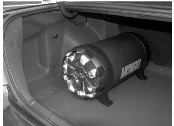
In a sedan: the tube should be secured against the sides of the trunk, firing toward the rear of the vehicle.
